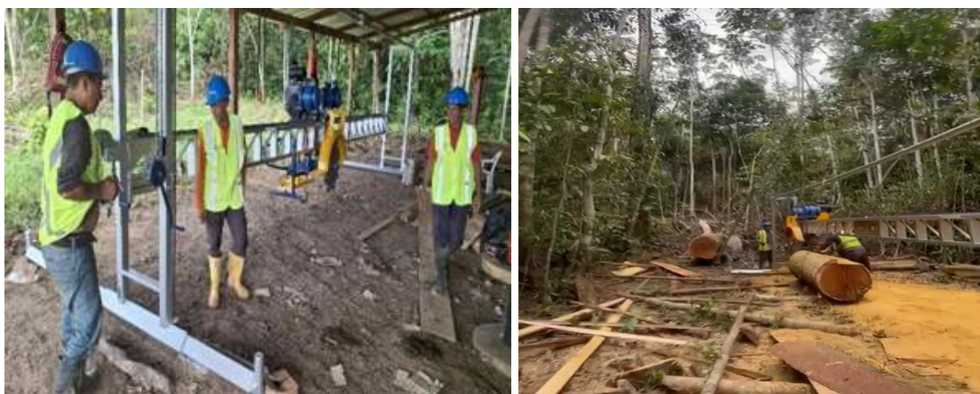
Figure 9. Installation and operation of the Vectron 3530 portable sawmill
